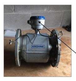
This is a Remote Head Flowmeter with Wire Junction Box, thereby removing delicate electrical equipment from a hazardous location and adverse weather conditions. See below for Signal Converter Head located in a safe place.
