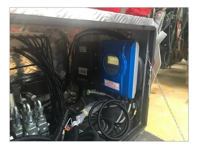
The Flowmeter Signal Converter has been mounted in a safe location on the chassis of the Tanker within a Control Box.
