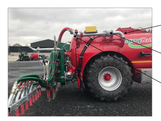
Discharge pipe rising internally – gate valve controlled.
