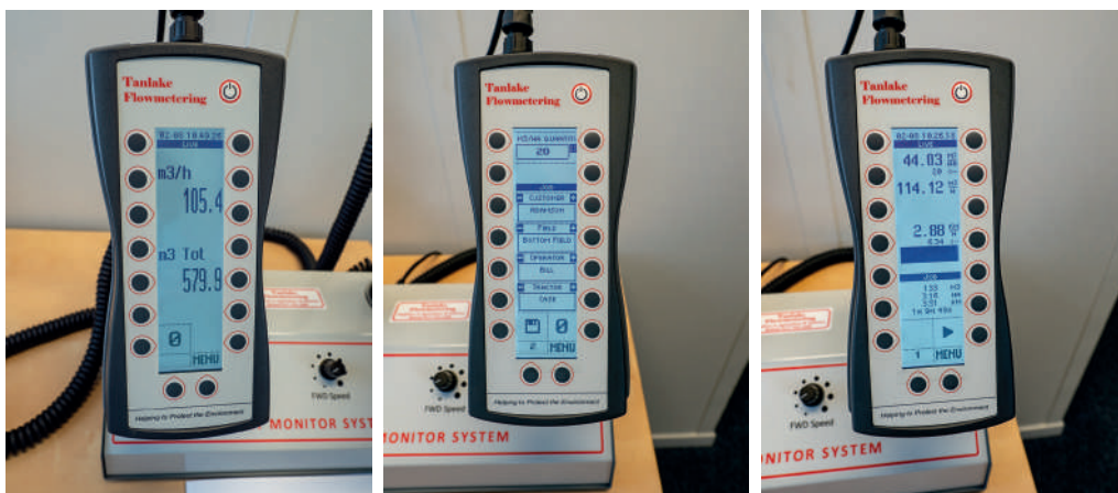
Developed specifically for slurry application, the latest Tanlake Flowmetering in-cab controls come in two forms; entry level and advanced. The former (left) has a single display menu and lists core details to include slurry flow rate and the total applied. This unit is ideal for the farm user where the size of fields are known. For greater data recording and more advanced monitoring, the second monitor system has two core menus, the first details raw data to include customer and field details, where the material is applied and the name of the operator. The second menu displays forward speed, flow rate and application data in cubic metres per hectare. All information can be downloaded via a USB port onto purpose built office software.
